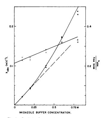
Fig. 5.—Catalysis of *p*-methylphenyl acetate hydrolysis by imidazole buffer, 90% free base, pH 8.25, at 25°, ionic strength 1.0, 0.1 *M* sodium arsenate; left scale is for lower lines; dashed line calculated for rate law dependent upon first-order term in imidazole only; upper line and right scale,  $k_{obsd}$ /[free amine].
