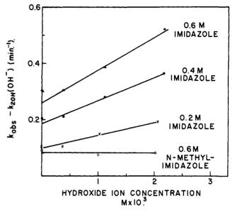
Fig. 2.—Imidazole-catalyzed hydrolysis of phenyl acetate,  $k_{obsd} - k_{20H}^{-1}[OH^{-}]$ , in 0.15 *M* triethylamine buffers at 25°, ionic strength 1.0. The points on the ordinate are calculated from values of  $k_1$  of 0.52  $M^{-1}$  min.<sup>-1</sup> for imidazole<sup>19</sup> and 0.15  $M^{-1}$ min.<sup>-1</sup> for N-methylimidazole;  $k_{OH}^{-} = 76 M^{-1}$  min.<sup>-1</sup>.
