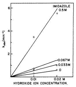
Fig. 1.—Imidazole-catalyzed hydrolysis of p-nitrophenyl toluate in alkaline solution in 30% acetonitrile at  $25^{\circ}$ .
