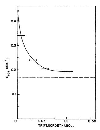
Fig. 4.—Observed pseudo-first-order rate constants for the hydrolysis of trifluoroethyl acetate in 0.75 M imidazole at pH 11.00  $\pm$  0.02, determined by automatic titration. The horizontal lines represent the range of trifluoroethanol concentration produced by hydrolysis of the ester during the experiment. The dashed line is the uncatalyzed alkaline hydrolysis rate at pH 11.00.<sup>19</sup>
